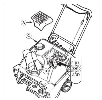
Figure 9. Add / Check Engine Oil and Gasoline
